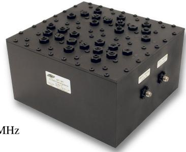
EWT-12-0235 is from a family of filters and duplexers designed for LTE applications. Featuring low IMD products, this model has passband frequencies of 791-821 MHz and 832-862 MHz and exhibits typical passband insertion loss of 1.25 dB with passband return loss of 20 dB. The co-channel isolation is > 60 dB.
